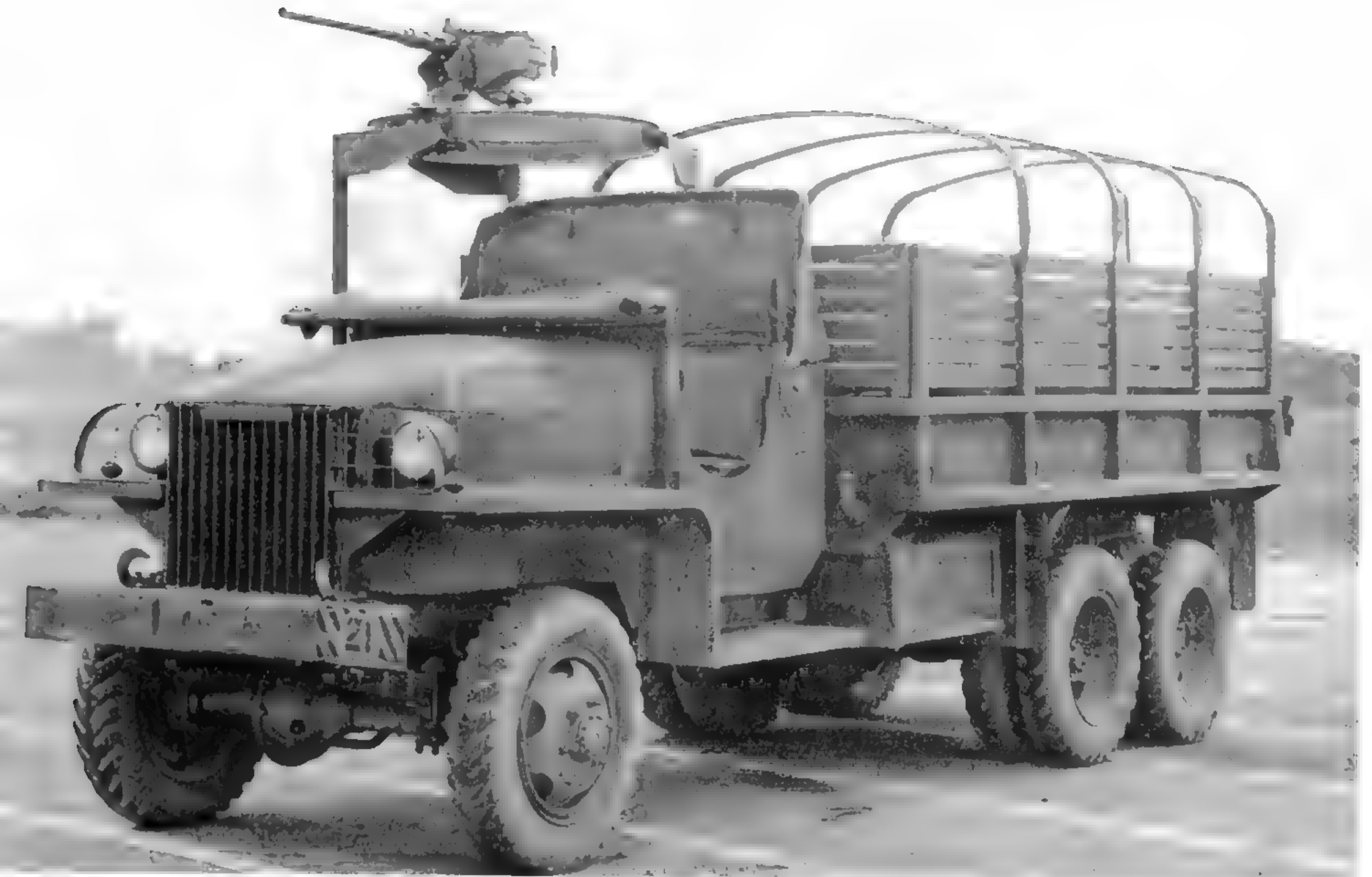
While Studebaker developed what was to become the military standard open cab, only a few of the US6s were built with the open cab. The biggest user of the US6, Russia, preferred the closed cab. Open-cabbed US6s are very rare today in the U.S. (National Archives photo)
